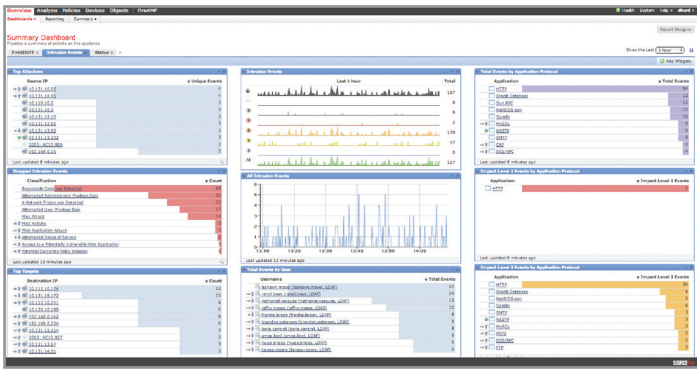
Figure 6-1: Sourcefire dashboard displays correlated intrusion events by severity
